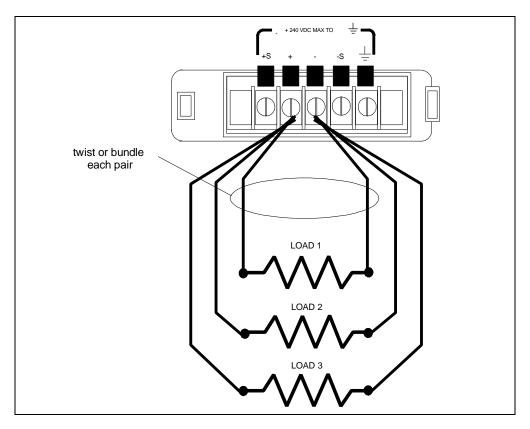
Figure 3-2. Multiple Load Connections
