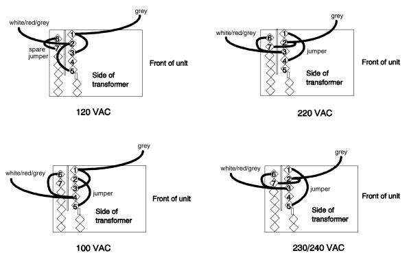
Figure D-1, Power Transformer AC Input Connections
