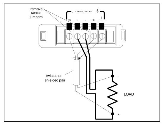
Figure 3-3. Remote Sense Connections
