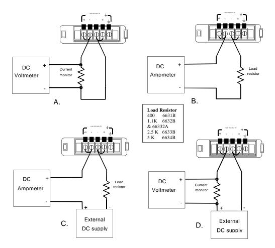
Figure B-1. Verification & Calibration Test Setup
